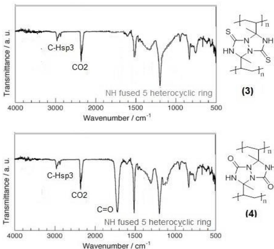
Figure 1. IR spectra of polymers (**3**) and (**4**)
