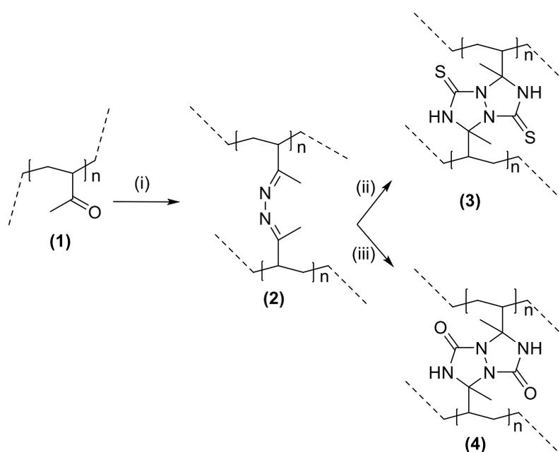
Scheme 1. synthesis of 2, 3 and 4 polymer.(i) NH<sub>2</sub>-NH<sub>2</sub> (ii) KSCN, CH<sub>3</sub>COOH, (iii) KNCO, CH<sub>3</sub>COOH
